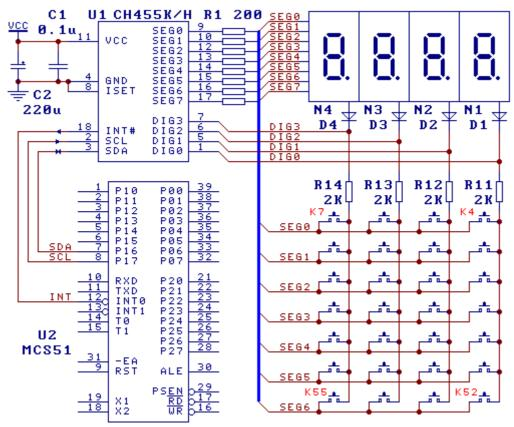
8.2. Drive common anticathode numeric LEDs (following image)
