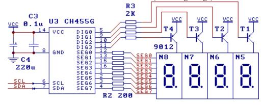
After adding reversers in DIG0~DIG3 word pins, CH455 can drive common anticathode numeric LEDs. In the image, the reversers are composed of four PNP audions T1~T4 (type of 9012 or 8550) and four resistors R3 (1K $\Omega$  to 3K $\Omega$ ), drive four common anticathode numeric. The SEG segment is converse drive in this connection, so the word data in load word data command
